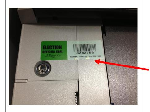
Remove the sticker seal from the access door by the printer.
