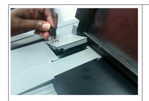
Close and lock compartment with barrel key.
