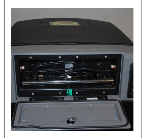
Wrap cord neatly, using the Velcro that's attached to the cord and place back in the compartment
