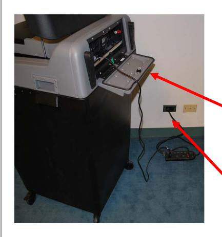
Unlock wheels and turn the DS200 around. Using silver key, unlock the back door compartment.
